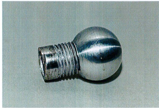
Fig. 8: Cementing cap with a screwed on load attachment.
